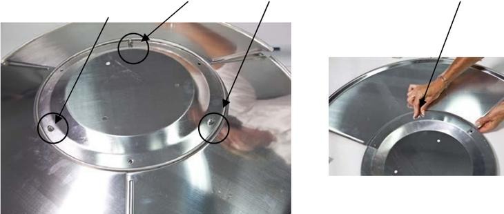
Next, align the sides of each outer piece and the center piece and insert the next 3 bolts through both holes. Tighten castle nuts on bolts.
