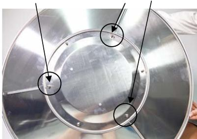
Finally, insert bolt through holes located at outside edge of adjoining panels of the reflector side pieces (3 bolts required) and tighten castle nuts on bolts.
